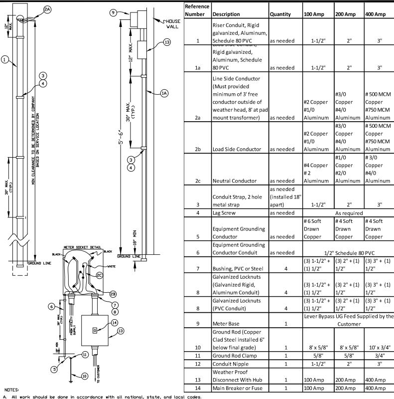
B. Line and Load side neutral conductors must be clearly marked with white tape.
